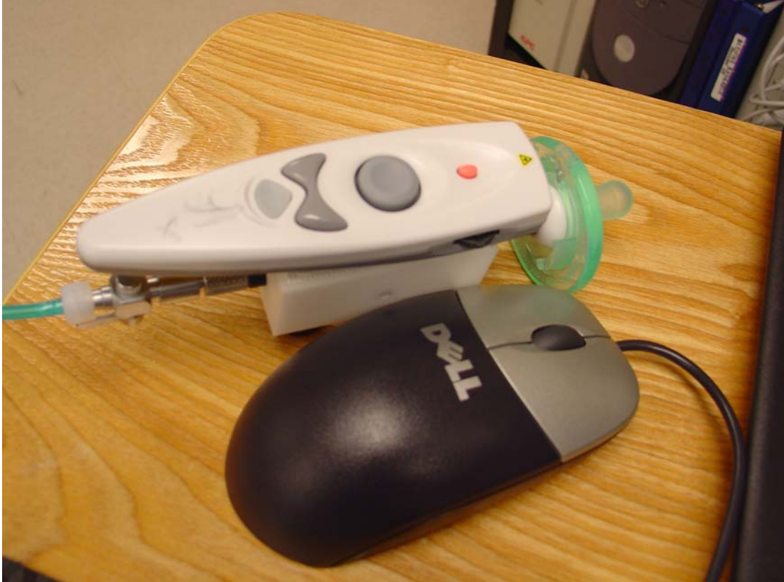
Figure 16. Remote control for NTrainer RT – Wireless Mouse, and regular mouse. User could control NTrainer by both of them
